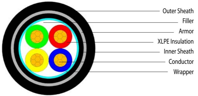
**Rated voltage: 0.6/1kV-four core**
