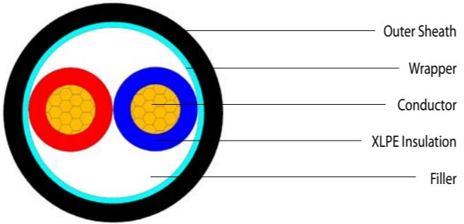
**Rated voltage: 0.6/1kV-two core**
