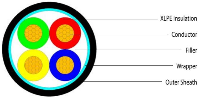
**Rated voltage: 0.6/1kV-four core**
