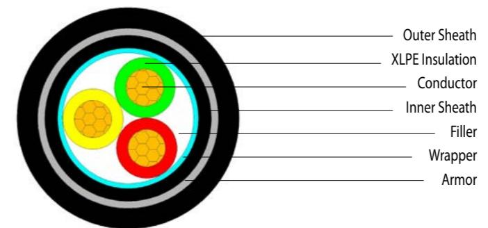
**Rated voltage: 0.6/1kV- three core**
