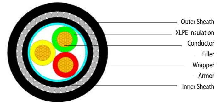
**Rated voltage: 0.6/1kV-three core**
