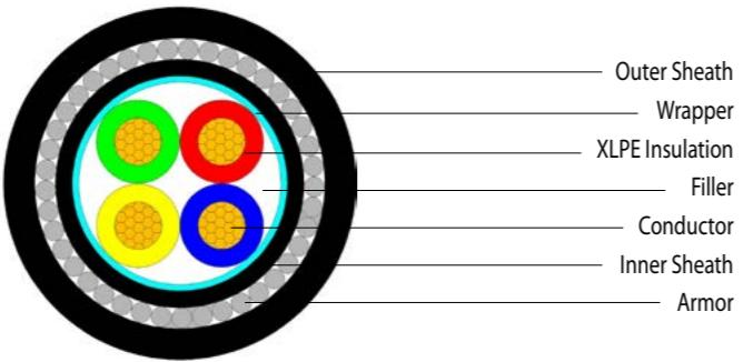
**Rated voltage: 0.6/1kV-four core**
