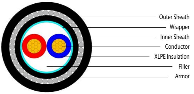
**Rated voltage: 0.6/1kV-two core**
