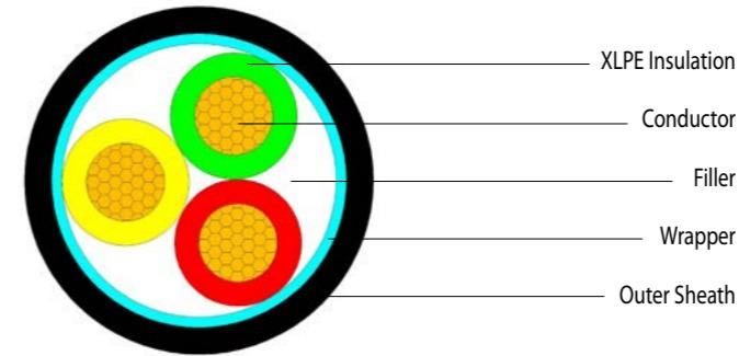
**Rated voltage: 0.6/1kV-three core**
