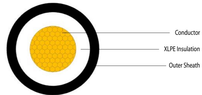
**Rated voltage: 0.6/1kV-single core**
