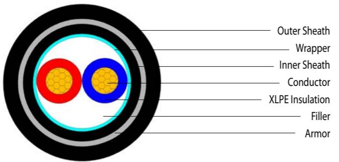
**Rated voltage: 0.6/1kV- two core**
